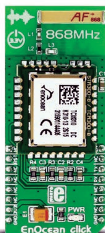
EnOcean sensor module used in building automation
